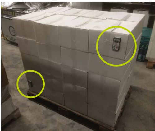
Positioning of outside loggers on the pallet
