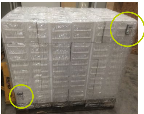
Positioning of outside loggers on the pallet
