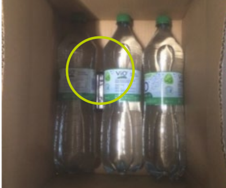
Positioning of inside logger inside the cardboard box
