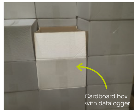
Positioning of inside logger on pallet
